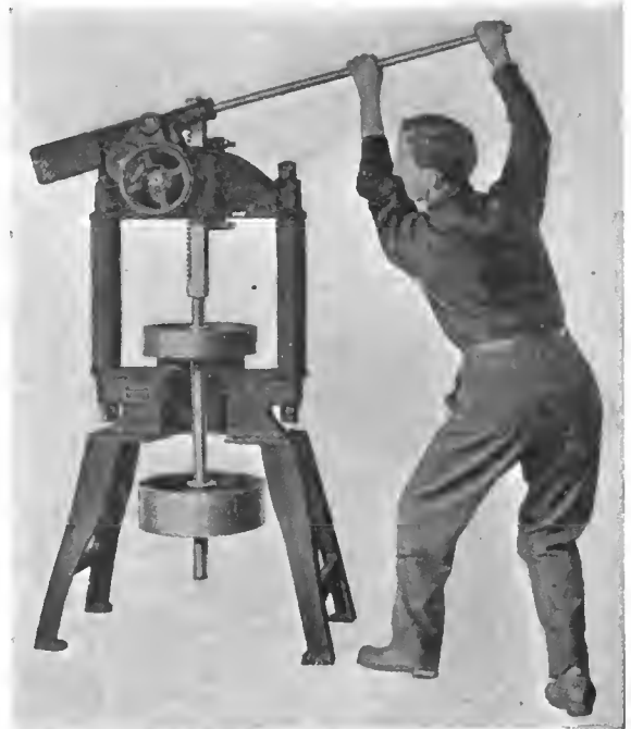
At the left is illustrated the Battle Creek steam vulcanizer for the repair of casings or tubes. Six casings and several tubes may be treated at one time
